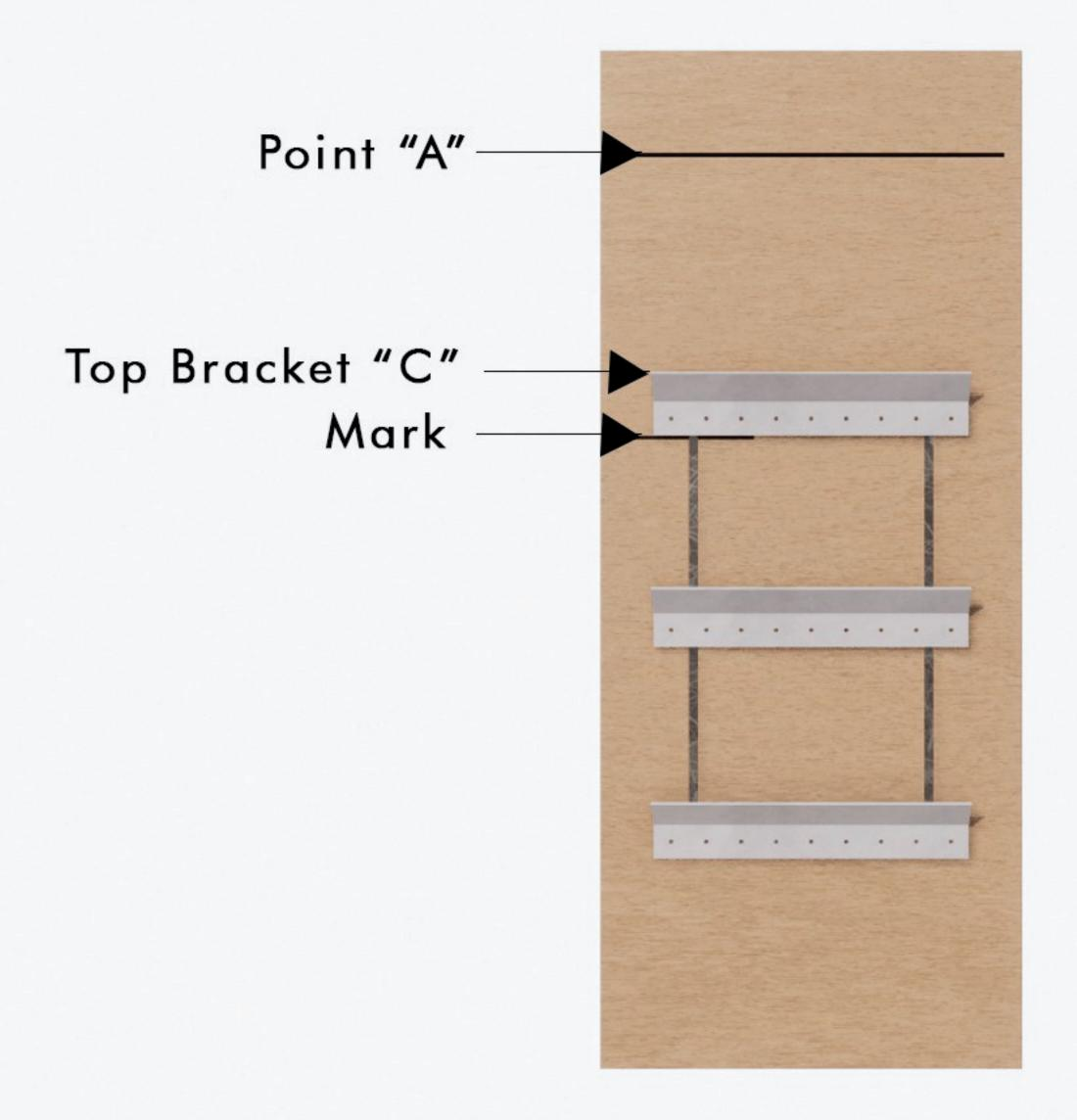
3. Place the bottom of top bracket "C" on the mark and mount with specified fastener. See Detail E.
