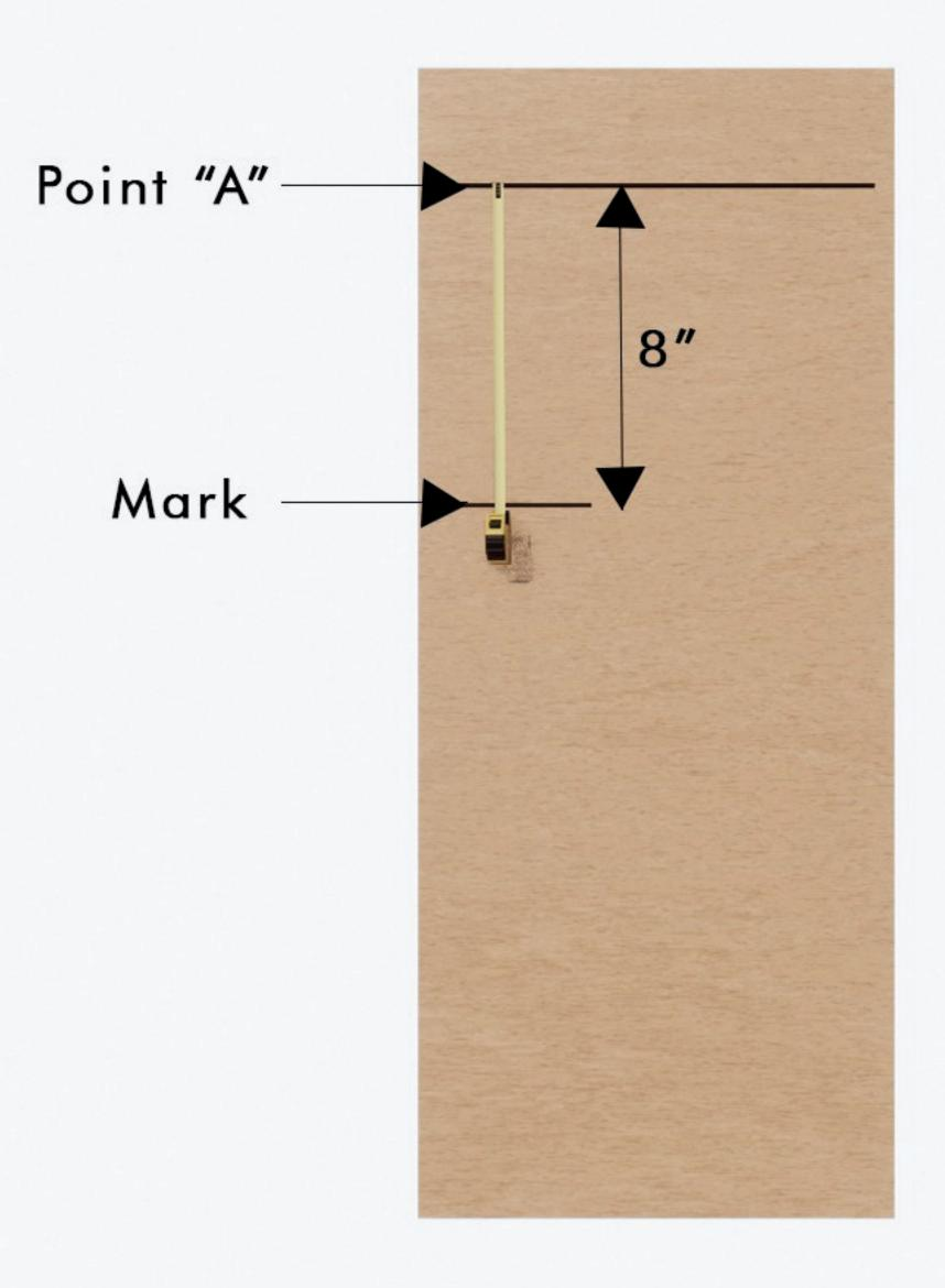
2. Measure 8" down from point "A" and mark the wall.
