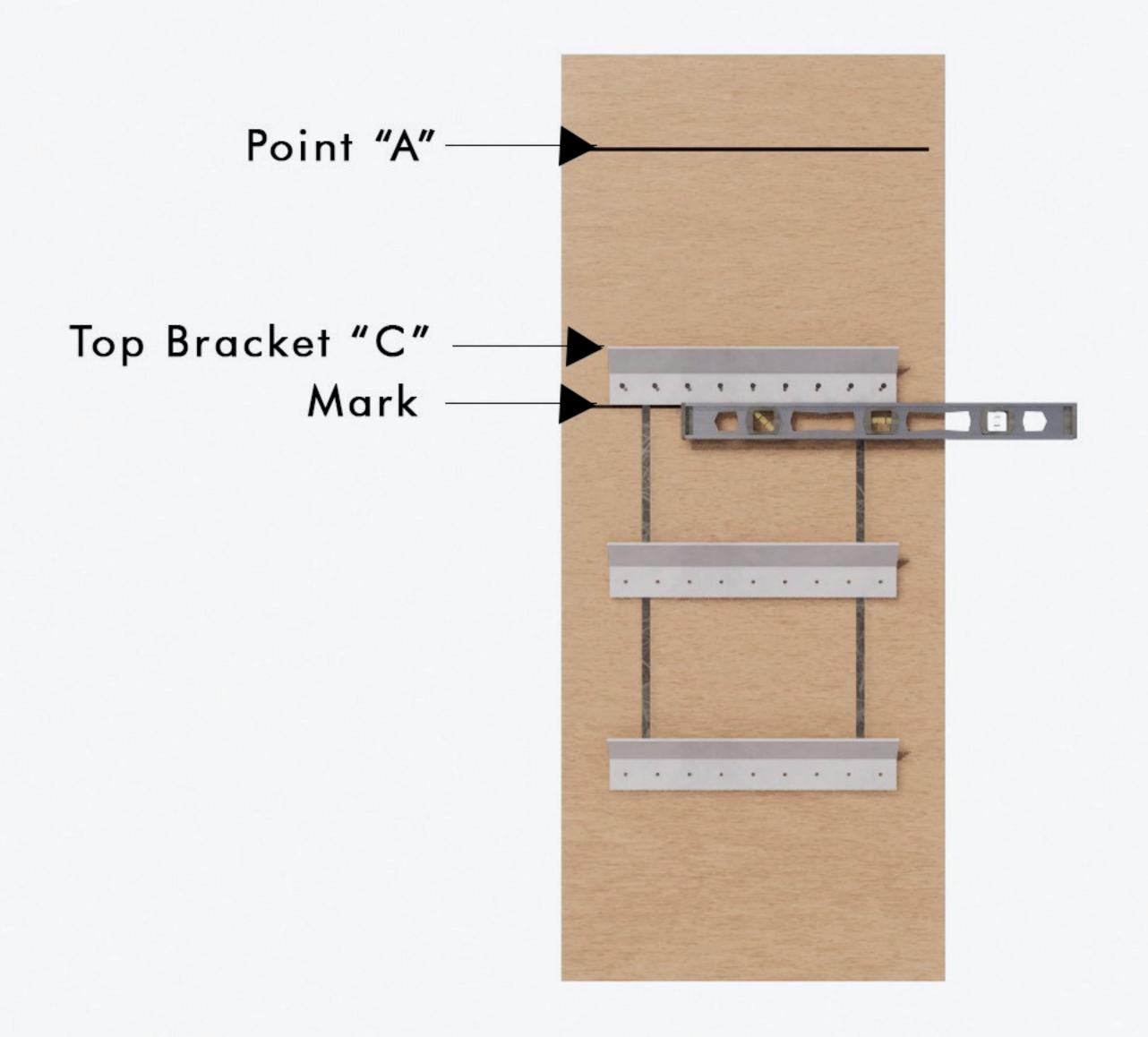
4. Level Bracket "C." Install fasteners in pre-drilled holes.
