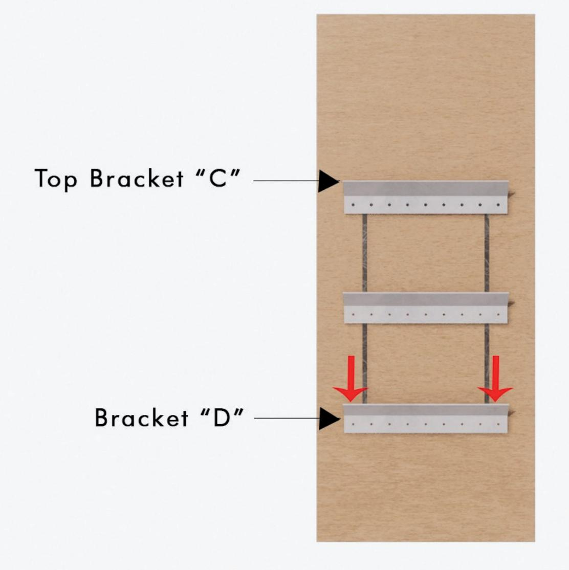
5. Once bracket "C" is secure, put slight pressure on bracket "D" ensuring banding is tight.
