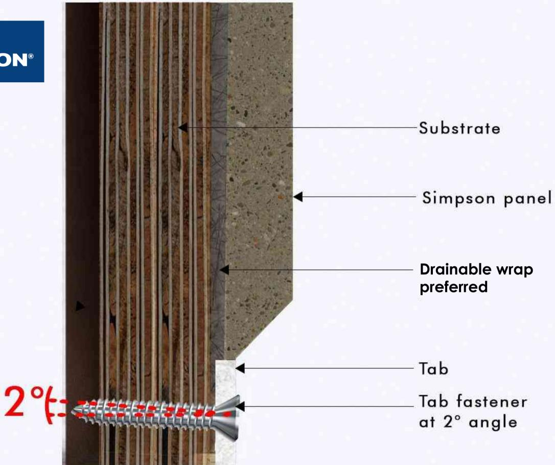
Install specified fastener (see Figure "C") in tab on a slight 2° angle and flush head of fastener.
