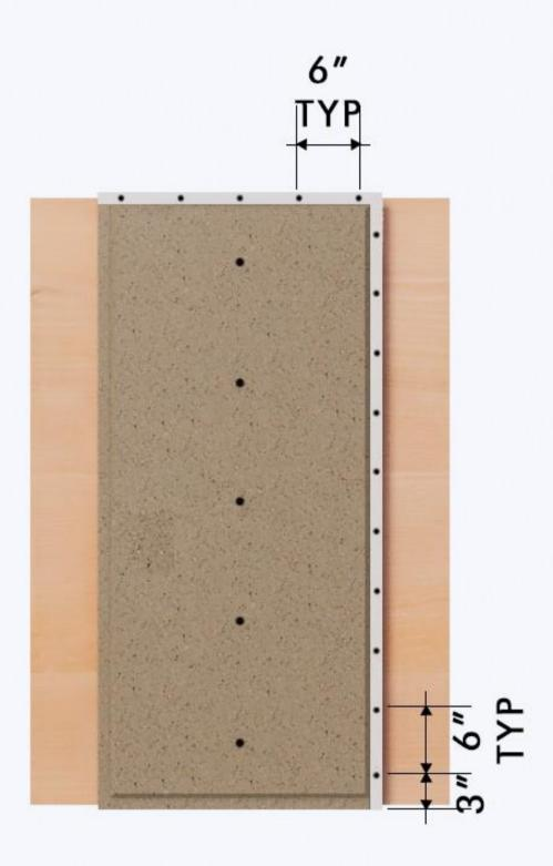
4. Install specified fasteners in tab 3" from ends and spaced evenly every 6".
