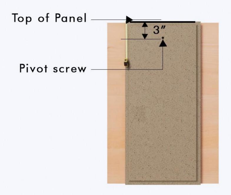
2. Place top of panel on mark and install pivot anchor 3" from the top edge. See figure "B".
