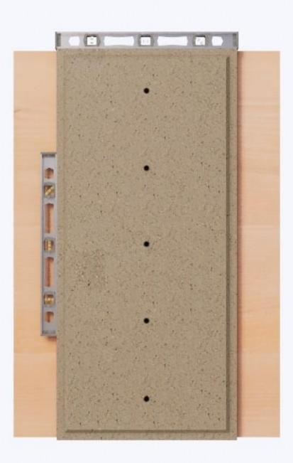
3. Level panel vertically and install remaining infield fasteners. See figures "A" and "B."
