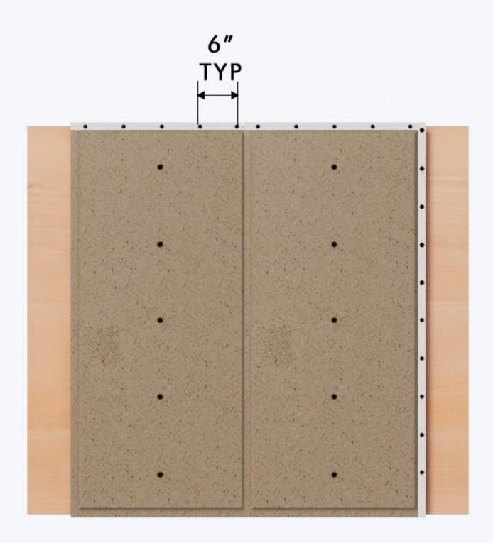
5. Install the second panel by installing it snug to the first panel and install screws at the tab and at the pivot but not at the finished edge where the panel adjoin.
